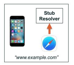
The phone's stub resolver sends a query for *www.example.com*, IN, A to 4.2.2.2
